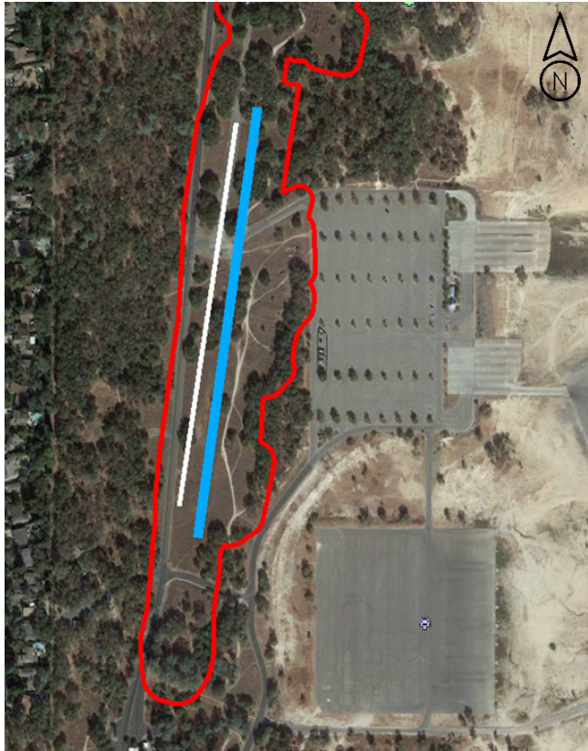
Figure 2-1. Existing Dike 3 Centerline (White), Proposed New Dike 3 Centerline (Blue and 80ft closer to Folsom Lake), and the Area of Potential Effects (Red).
